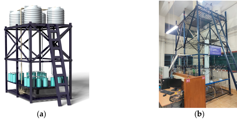
Figure 1. (a) Three-dimensional model of RTCOP-WDN setup; (b) a fully functional RTCOP-WDN test facility.
