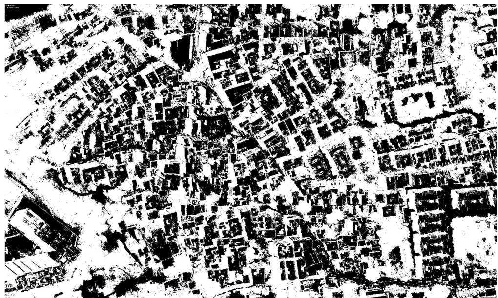
Figure 5. After corrections, and applying the 'Threshold' filter, the image is converted into a binary black-and-white pattern.
