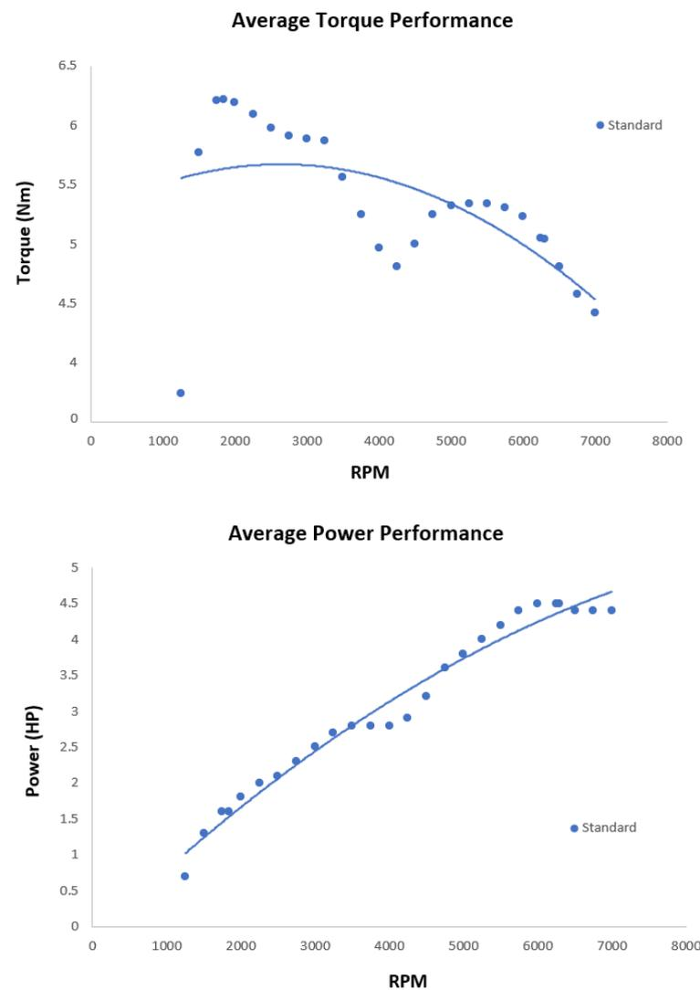
Figure 3. Engine torque and power performance graph without HHO generator.
