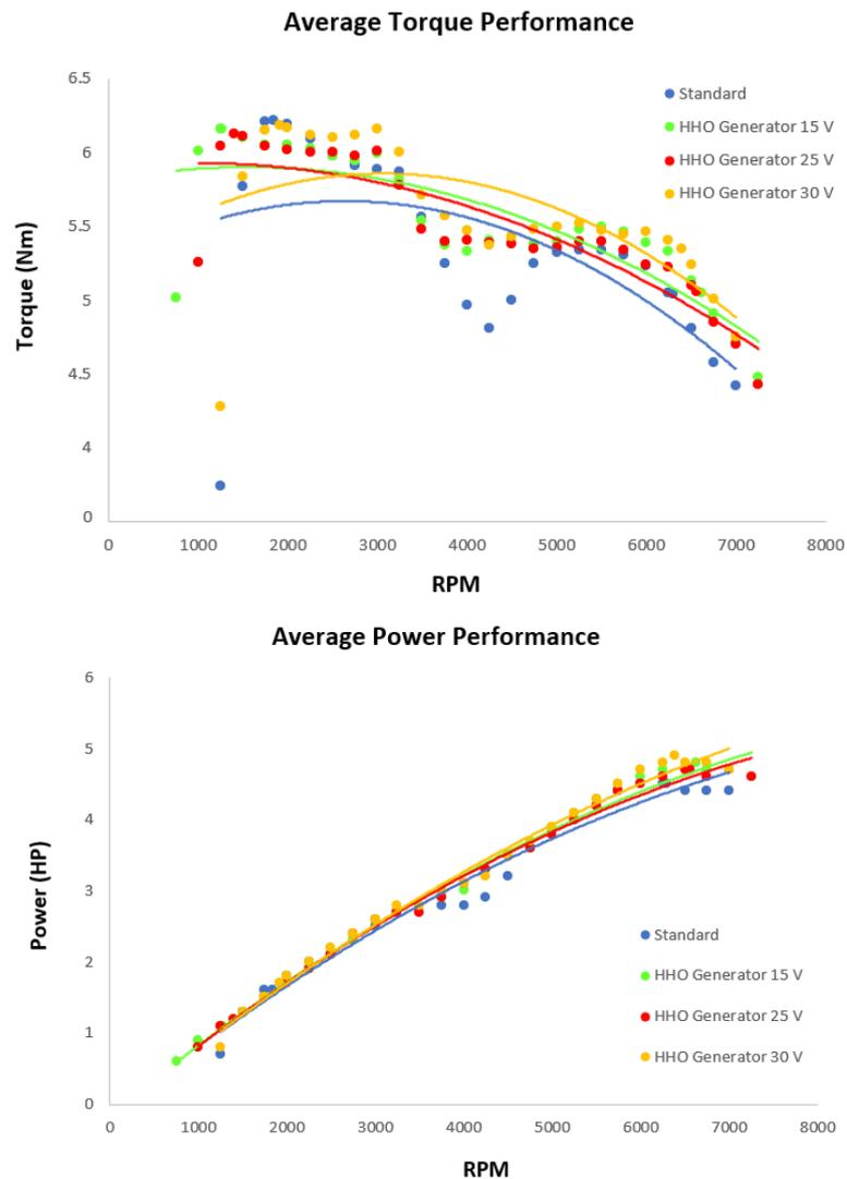
**Figure 4.** Engine torque and power performance graph with and without HHO generator.
