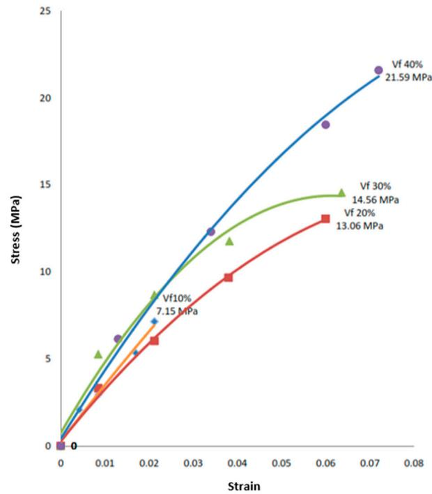
**Figure 3.** The Relationship between Stress and Strain at Varying Volume Fractions of 10%, 20%, 30%, 40%.
