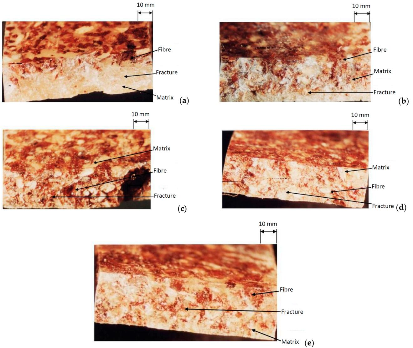
**Figure 7.** Cross section macro photo of tensile test specimen  $V_f = 10\%$  (a),  $20\%$  (b),  $30\%$  (c),  $40\%$  (d) and  $V_f = 50\%$  (e).
