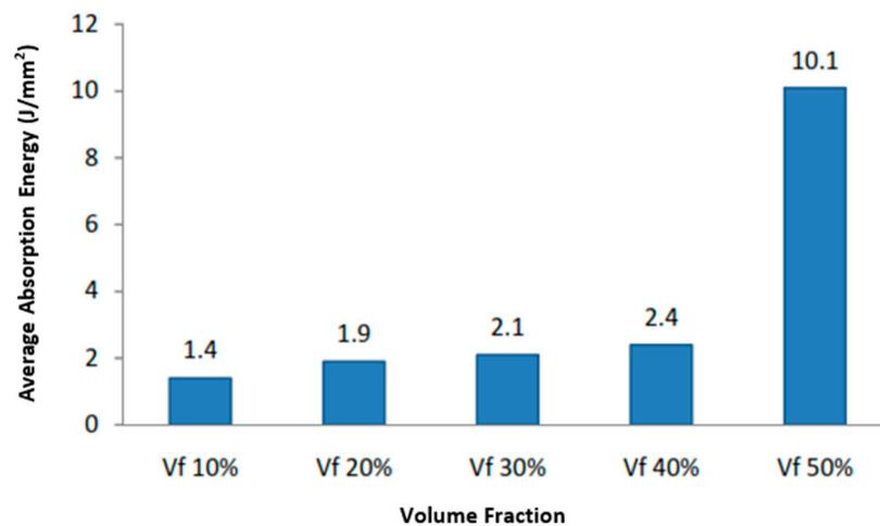
**Figure 4.** Histogram of the Average Absorption Energy of Coconut Shell Composite with Epoxy Matrix at a Particle Diameter of 1 mm.
