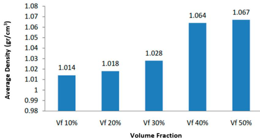
**Figure 6.** Histogram of Average Density of Coconut Shell Composite with Epoxy Matrix at a Particle Diameter of 1 mm.
