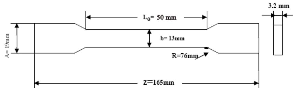
Figure 2. Tensile Test Speciment Geometry.
