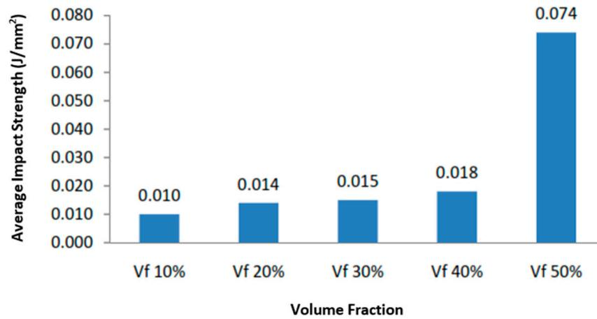
**Figure 5.** Histogram of Average Impact Strength Values for Coconut Shell Composite with Epoxy Matrix at a Particle Diameter of 1 mm.
