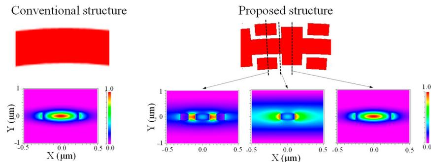
**Figure 2.** Electric field intensity distribution  $E_x$  of the conventional structure and the proposed structure.
