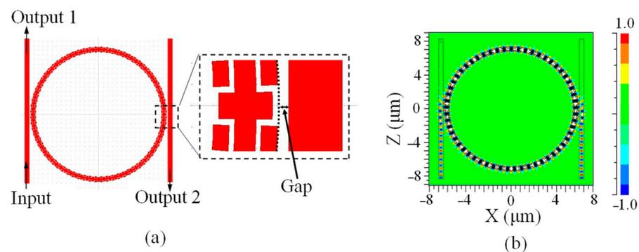
**Figure 4.** (a) Structure of proposed micro-ring resonator biosensor. (b) Magnetic field distribution  $H_y$ .
