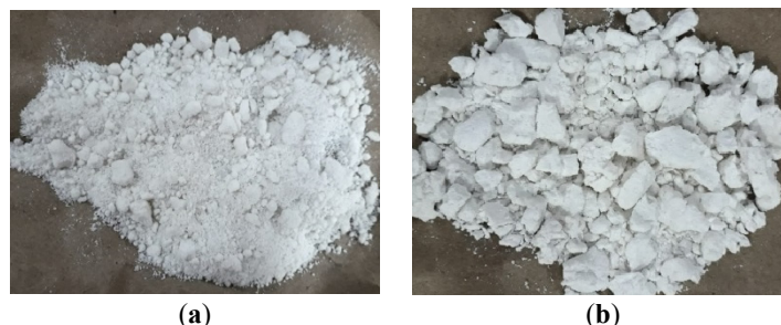
Figure 9. Struvite with the following compositions: (a) product A with a molar ratio of \text{PO}_4^{3-}:\text{Mg}^{2+}:\text{NH}_4^+ = 1: 1.5: 2 ; (b) product B with a molar ratio of \text{PO}_4^{3-}:\text{Mg}^{2+}:\text{NH}_4^+ = 1: 2: 4 .
