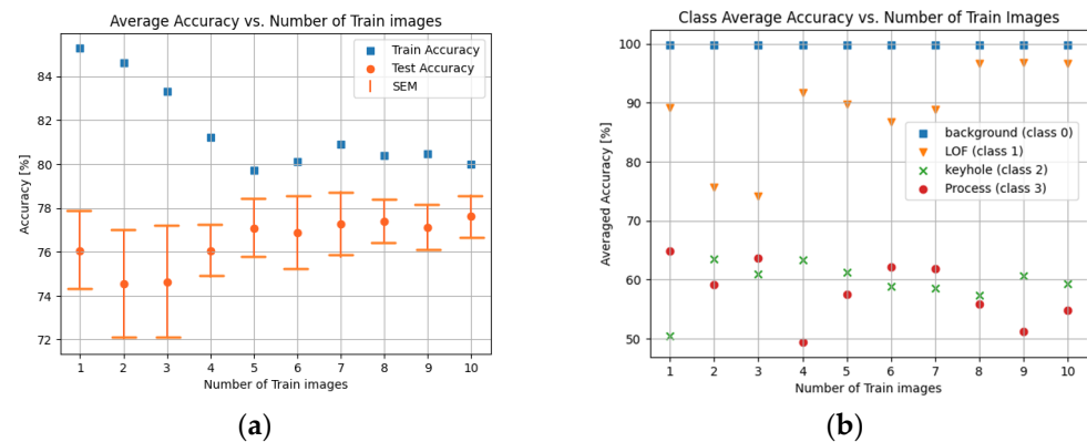
Figure 5. Figure 5. (a) Overall averaged accuracy of RF classifier vs. increasing number of training images, (b) each class-averaged accuracy of RF classifier vs. increasing number of training images.
