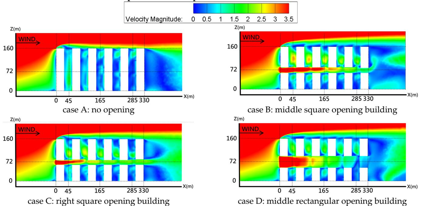
**Figure 3.** Profile of wind speed simulation results.
