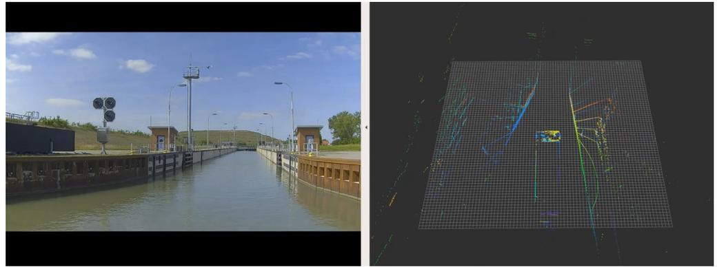
**Figure 6.** Screenshot of LiDAR and camera data during lock entry.
