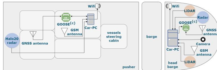
**Figure 2.** The hardware architecture on the test vessel. Sizes are not to scale.
