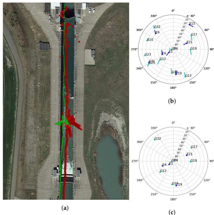
**Figure 5.** (a) L1/E1-based PVT solution (red) vs. Galileo E5a-based PVT solution (green), (b) skyplot during the whole cruise in the lock, (c) skyplot for the entire duration when the vessel is at the bottom and moves out of lock, Gx for GPS satellites (green) and Ex for Galileo satellites (blue).
