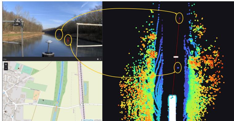
**Figure 8.** Three-dimensional pointclouds showing buoys in the canal.
