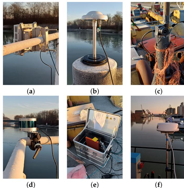
**Figure 4.** The sensor setup on the head barge, (a) Symeo radar, (b) GNSS antenna, (c) camera, (d) LiDAR sensors, (e) control box with the PC and GOOSE© receiver, and (f) Halo20 radar.
