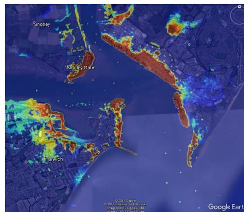
**Figure 3.** Radar conspicuity map of Harwich and Felixstowe, derived from the ship's radar and overlaid onto Google Earth. Hotter colours represent stronger, more reliable targets.
