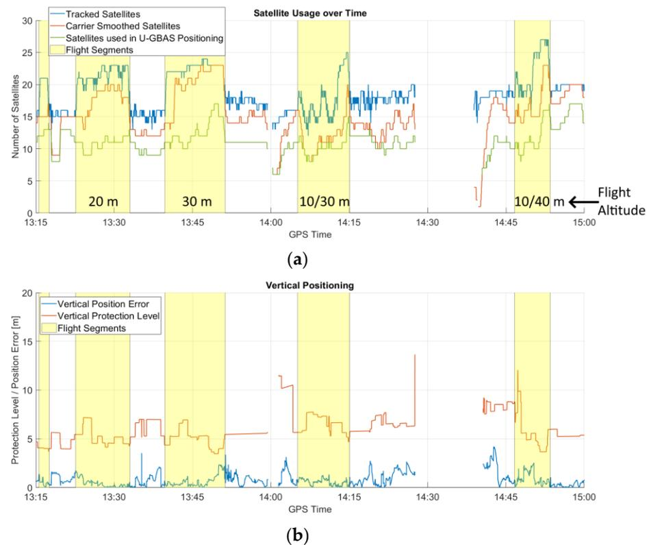
**Figure 5.** Results of flights between office buildings. (a) Satellite tracking and usage statistics during flights and on the ground; (b) achieved nominal ( $H_0$ ) protection level using a close-by reference station. Protection levels are derived for an L1/E1 100 s smoothing processing mode using GPS, Galileo and the nominal airborne noise model shown in Figure 4b.
