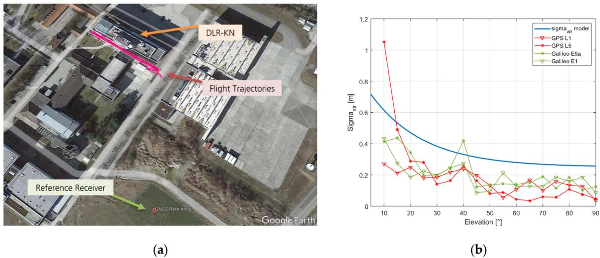
**Figure 4.** (a) Flight trajectories conducted in different heights (10–40 m) between two office buildings at the DLR campus Oberpfaffenhofen; (b) derived preliminary model for residual airborne noise and multipath ( $\sigma_{air}$ ) for 100 s code-carrier smoothing derived from around 4 h of GNSS measurements from the drone (blue) as well as measured residual errors over elevation for GPS and Galileo.
