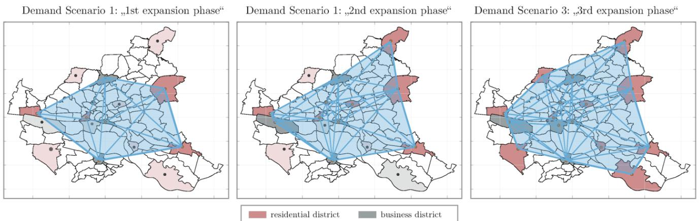
**Figure 1.** Assumed initial vertiport locations (black dots) for city of Hamburg based on a demand simulation. Figure adapted from [6]. The core service volume covered by the system is shaded in blue for each of the scenarios.
