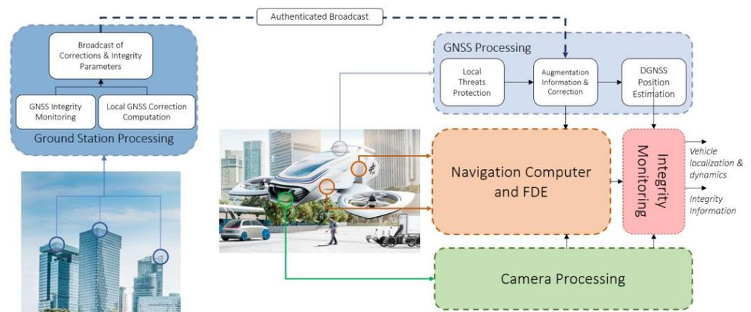
**Figure 2.** High-level system overview of the integration of the U-GBAS on ground within a multi-sensory onboard unit providing positioning as well as integrity information to the flight control system as well as air traffic management.
