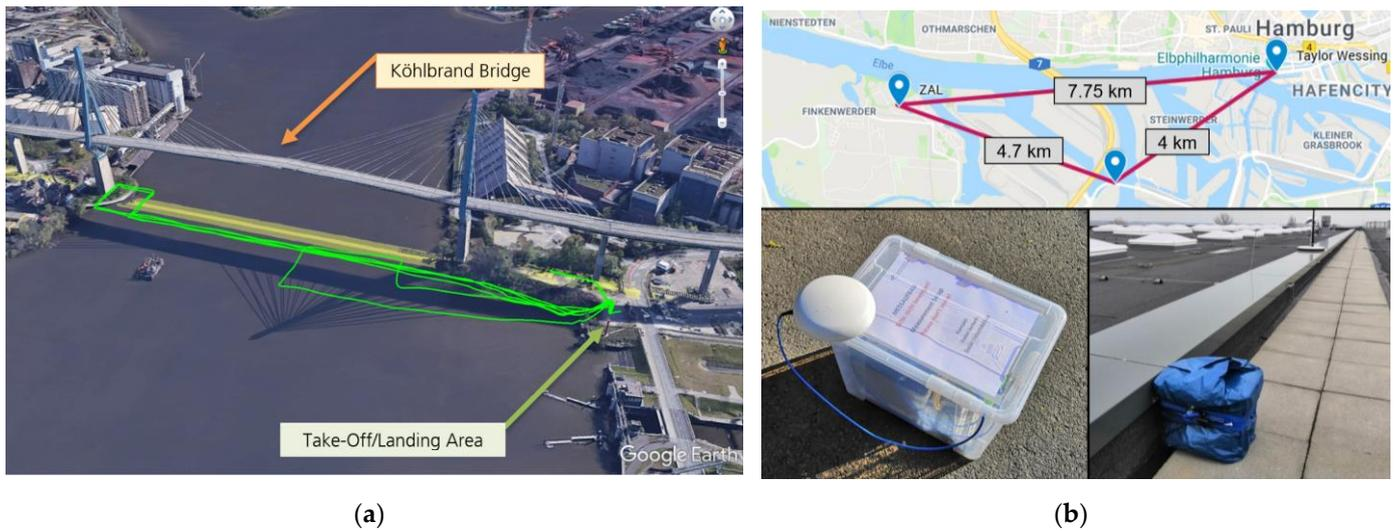
**Figure 3.** Flight trials in the city of Hamburg: (a) trajectory of the four flights conducted next to and below the bridge; (b) one of the three portable reference stations distributed across the city as shown in the map.
