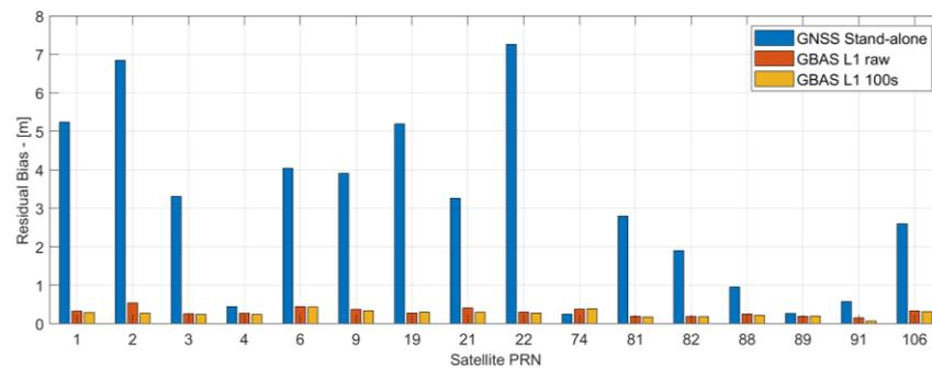
**Figure 6.** RMS error (bias) on ranges after application of corrections for the flight conducted in Hamburg.
