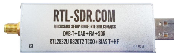
Figure 1. RTL-SDR (sixth generation) USB Dongle showing antenna connector (left) and USB port to connect with PC (right).
