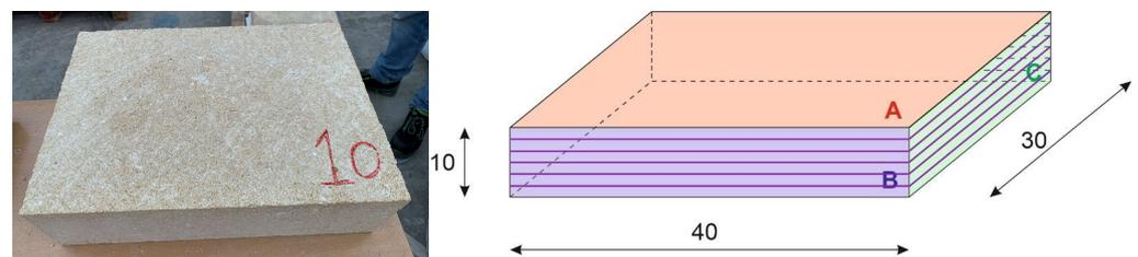
**Figure 1.** Ashlars provided by the quarry and assumed compression layers. Lengths in cm.
