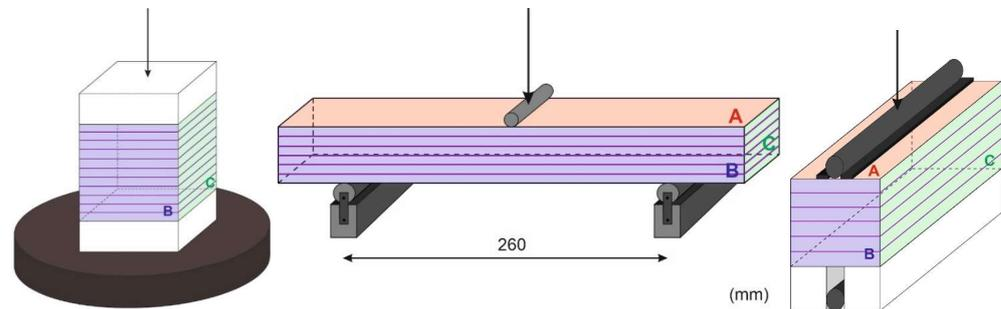
**Figure 2.** Test set ups for the uniaxial compression test (**left**), the three-point bending test (**middle**), and the split test (**right**). The arrow shows the loading direction.
