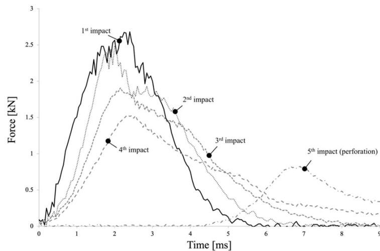
Figure 2. Force–time curves for the repeated low-velocity impacts.
