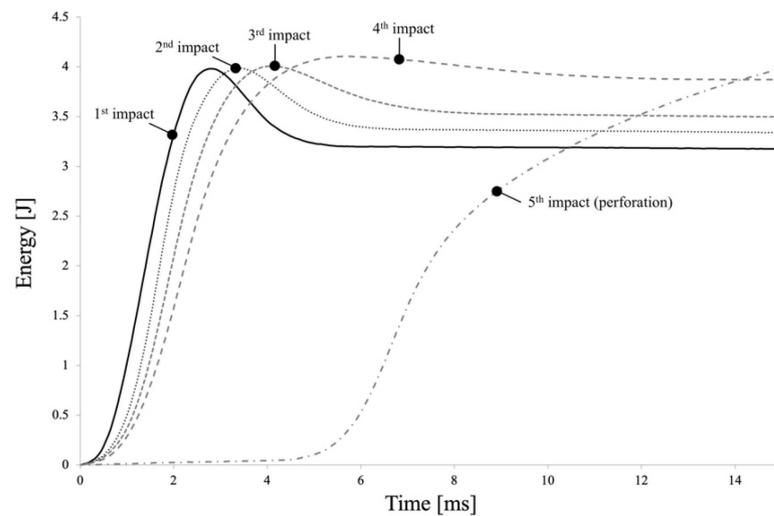
**Figure 4.** Energy–time curves for the repeated low-velocity impacts.
