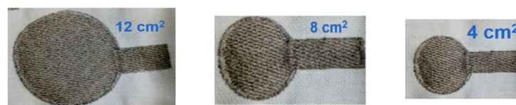
Figure 1. Developed ECG electrodes in different three sizes.
