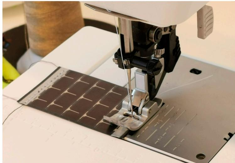
Figure 2. Stitching of flexible solar cells.
