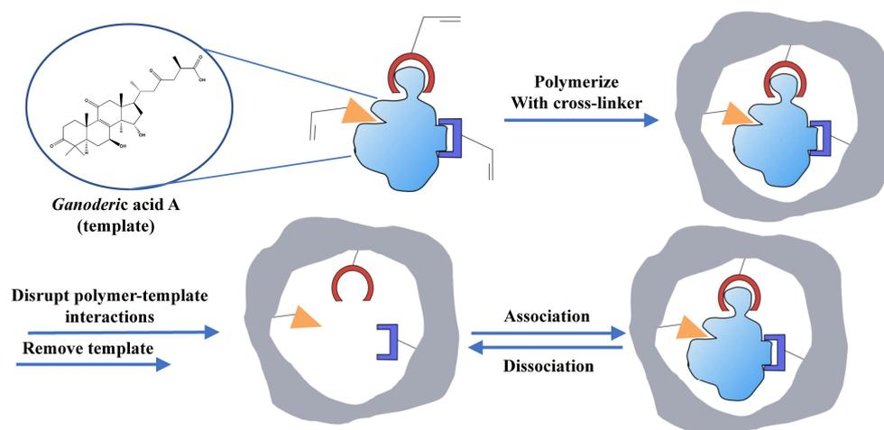
**Figure 2.** Schematic diagram of molecular imprinting principle of *Ganoderic acid A* as template.
