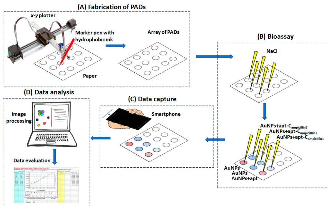
**Figure 2.** The experimental protocol for the fabrication of the PADS, the bioassay and data capture, analysis and evaluation.
