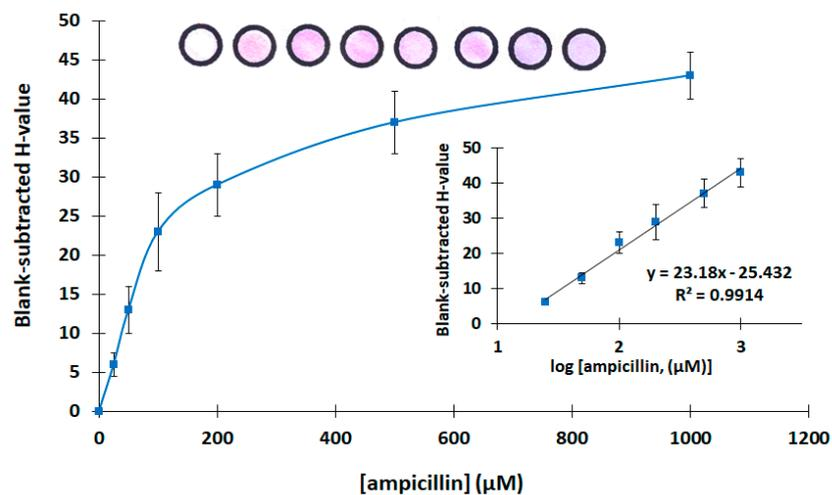
**Figure 4.** Calibration of ampicillin (the linear-log transformation of the calibration plot and photographs of the paper-based sensors at the different ampicillin concentrations are shown as inserts. The photograph at the left is a device with buffer only).
