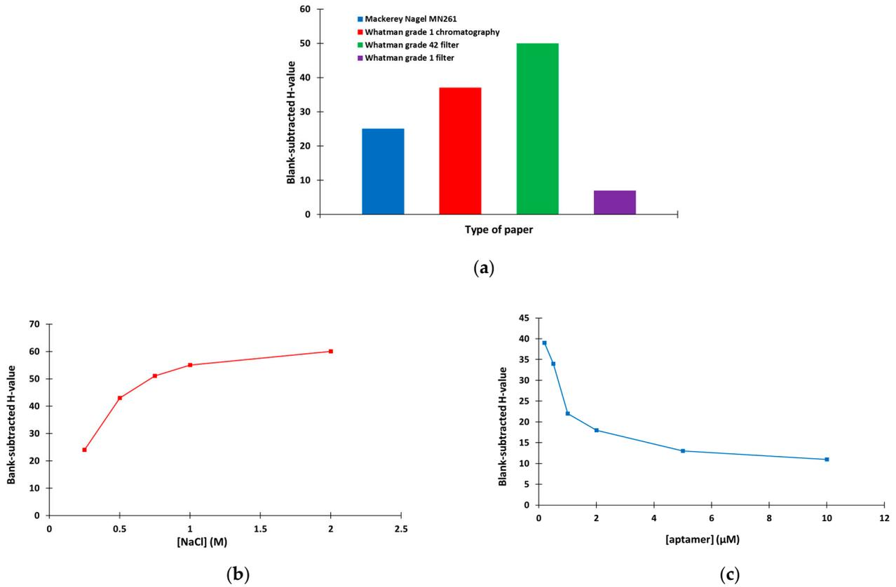
**Figure 3.** Selection of (a) the type of paper (8  $\mu$ L of 13.3 mM AuNPs + 8  $\mu$ L of 1 M NaCl), (b) the concentration of NaCl (8  $\mu$ L of 13.3 mM AuNPs + 8  $\mu$ L of NaCl at Whatman grade 42 filter paper) and (c) the concentration of aptamer (different concentrations of aptamer diluted in 10 mM of phosphate buffer (pH 7.4) containing 2 mM of  $MgCl_2$  was incubated with 13.3 mM AuNPs for 1 h and applied to the paper-based device modified with 1 M NaCl).
