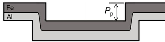
Figure 4. Schematic illustration of evaluation length as a joint deformation.
