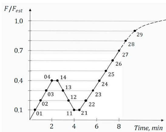
**Figure 6.** The standard loading procedure for monotonic loading [39].
