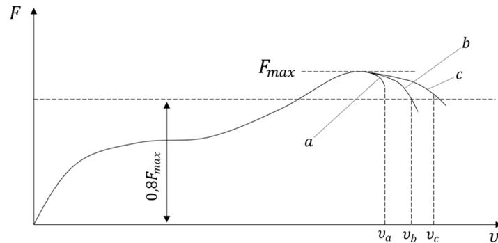
Figure 7. Definition of the ultimate force level for ductility according to the EN 12512 [40].
