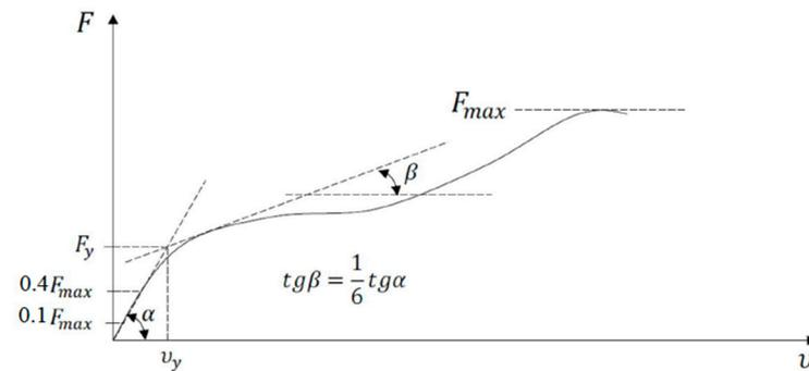
Figure 8. The so-called 1/6 method according to the EN 12512 [40].
