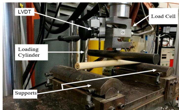
**Figure 3.** Experimental three-point bending tests set-up.
