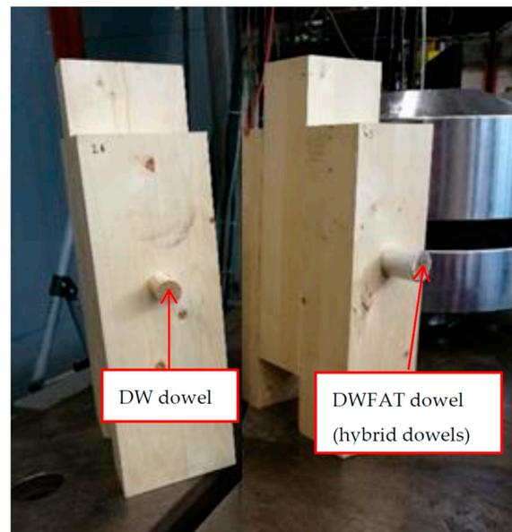
**Figure 10.** The different sets of tested timber-to-timber connections.
