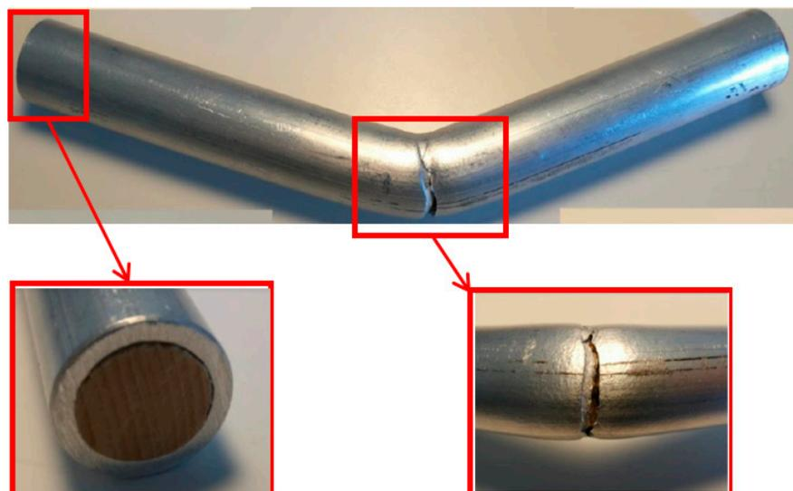
Figure 13. The main failure mode of the densified wood dowel filled aluminum tube (DWFAT) dowel.
