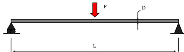
**Figure 2.** Three-point bending test scheme ( $L = 210$  mm).
