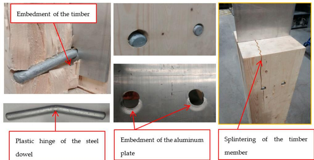
**Figure 17.** The main failure modes of slotted-in aluminum timber connections assembled using steel dowels.
