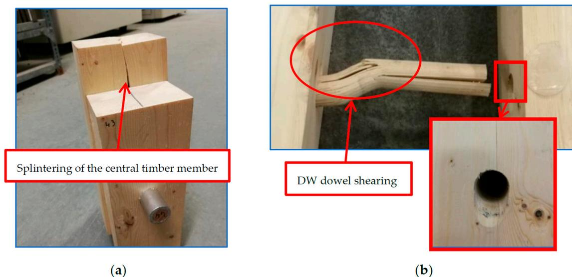
**Figure 15.** The main failure modes of push-out shear timber connections: (a) assembled using DWFAT dowels and (b) assembled using DW dowels.
