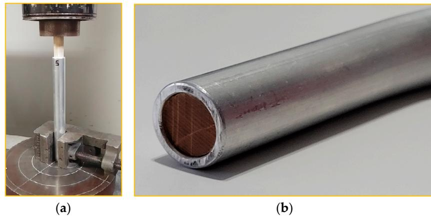
**Figure 1.** Densified wood-filled aluminum tube dowel: (a) manufacturing method, (b) prototype of hybrid dowel.
