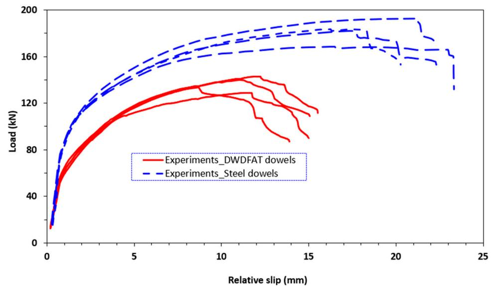
**Figure 16.** The load-slip curves for slotted-in aluminum plate timber connections assembled using steel or DWDFAT dowels.
