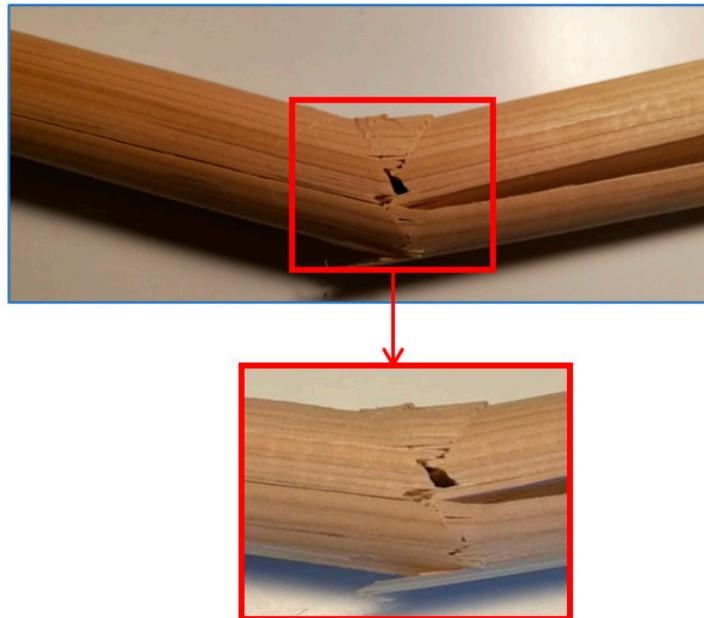
Figure 12. The main failure mode of the densified wood dowels (DWD).
