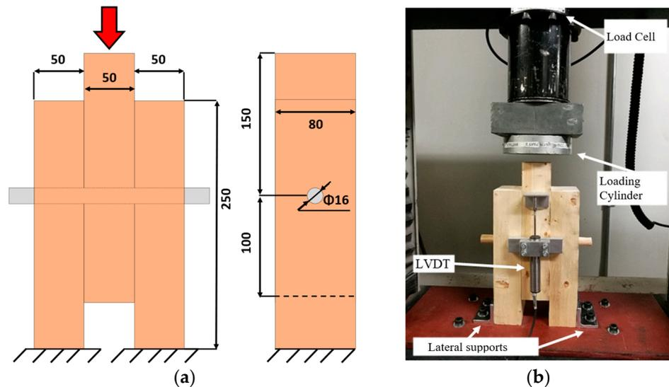
Figure 9. The push-out shear test: (a) geometrical description and (b) experimental set-up.
