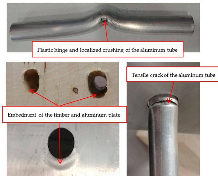
**Figure 18.** The main failure modes of slotted-in aluminum timber connections assembled using DWFAT dowels.
