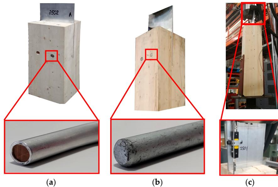
**Figure 5.** Experimental set-up of the slotted-in aluminum plate timber connection: (a) DWFAT dowel, (b) steel dowel and (c) experimental set-up.
