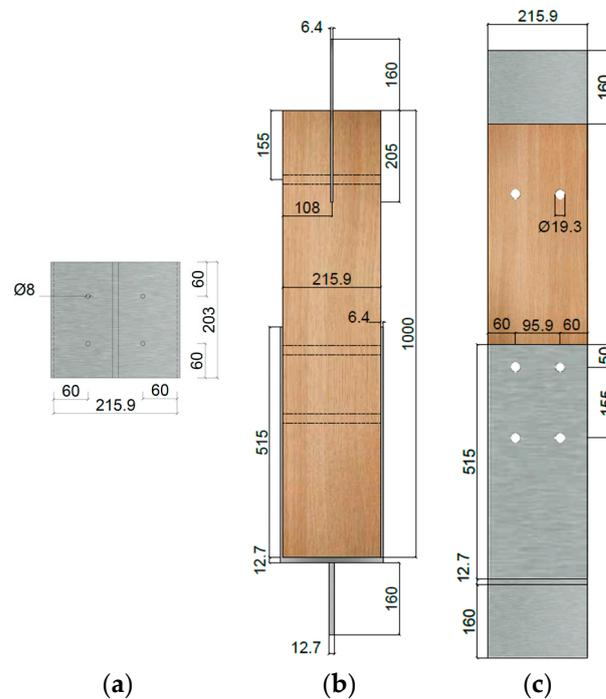
**Figure 4.** Geometrical description of the slotted-in aluminum timber connection: (a) bottom view, (b) front view and (c) side view.
