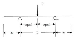
Figure 3. Beam with midspan load and overhangs.
