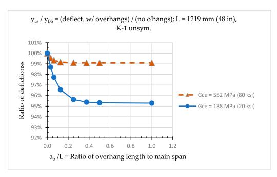
**Figure 5.** Deflection ratios for profile K-1 (not symmetric).
