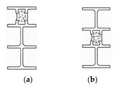
Figure 4. Profiles: (a) K-1 (unsymmetric); (b) F-1 (symmetric).
