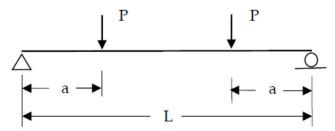
Figure 1. Beam with two symmetric loads.
