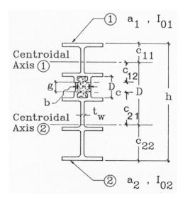
Figure 2. Example profile with geometric notation.
