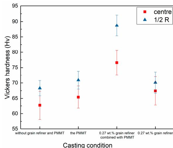
**Figure 5.** The Vickers hardness in different casting conditions.
