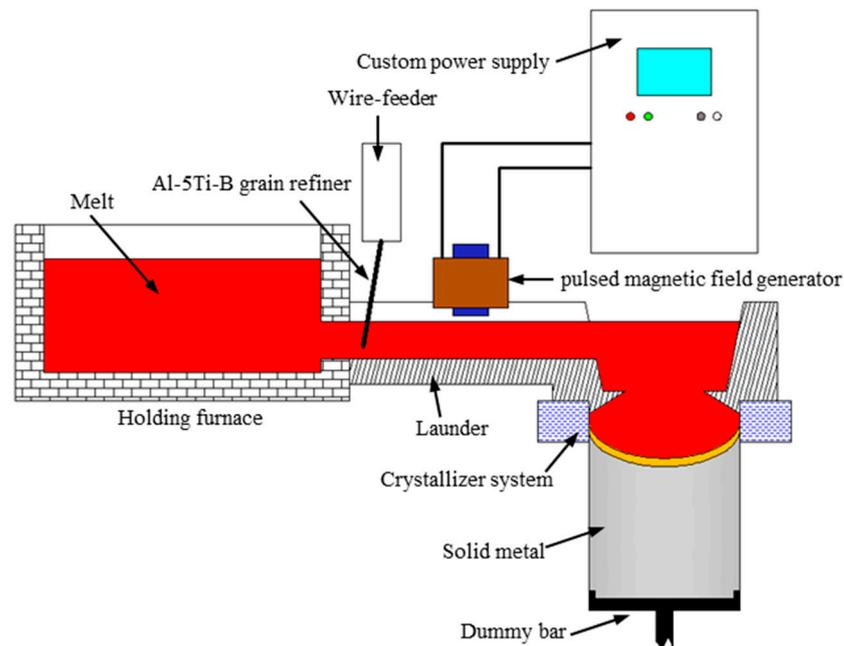
**Figure 1.** Schematic diagram of the device used in this study.
