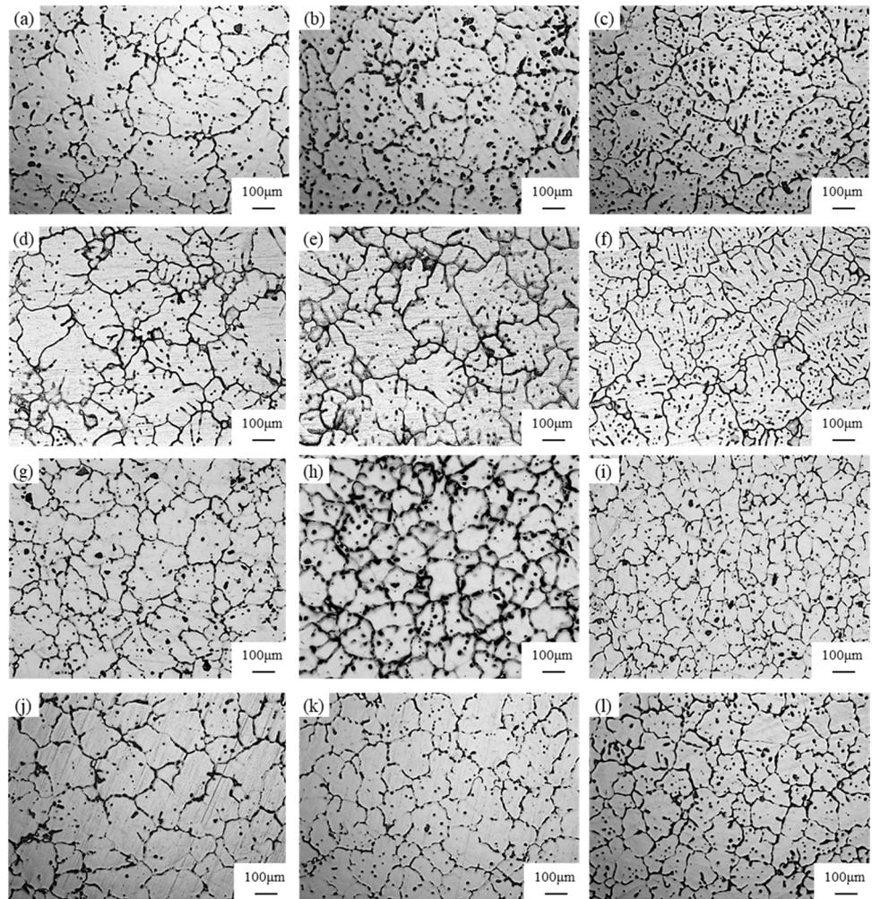
**Figure 3.** The microstructure of the billet under different casting conditions: without grain refiner and PMMT: (a) centre, (b) 1/2 R, (c) edge; the PMMT: (d) centre, (e) 1/2 R, (f) edge; 0.27 wt.% grain refiner combined with PMMT: (g) centre, (h) 1/2 R, (i) edge; 0.27 wt.% grain refiner: (j) centre, (k) 1/2 R, (l) edge.
