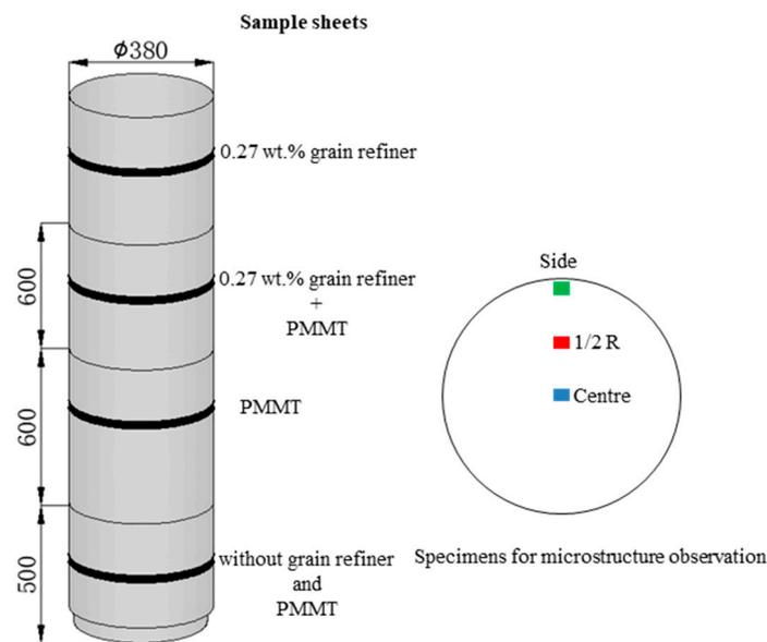
**Figure 2.** Schematic illustration of samples for microstructure observation.
