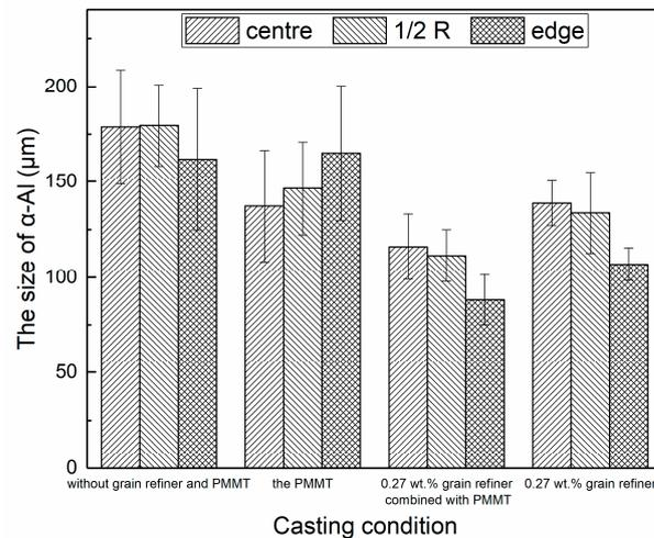
**Figure 4.** The size of  $\alpha$ -Al grains under different casting conditions.
