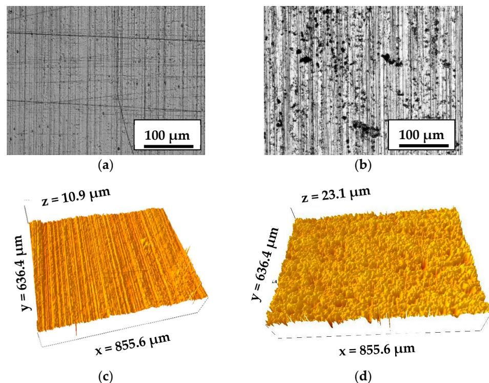
**Figure 1.** Optical images of as-received (a) PVC and (b) Al and their corresponding 3D profile images of the roughness in (c,d).
