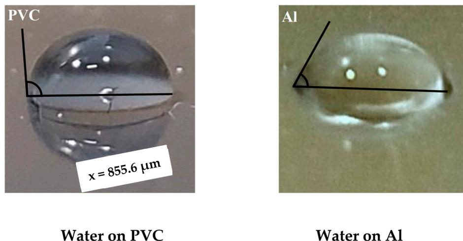
**Figure 2.** Digital image of a water droplet on the PVC and Al substrate surfaces showing the water contact angles.
