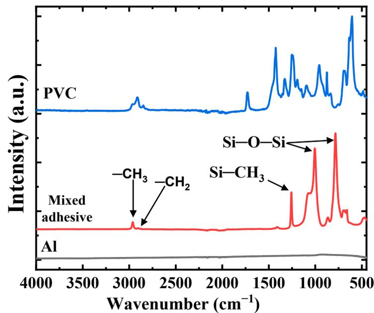
Figure 3. ATR-FTIR spectra of mixed adhesive of epoxy and silicone, PVC and Al surfaces.
