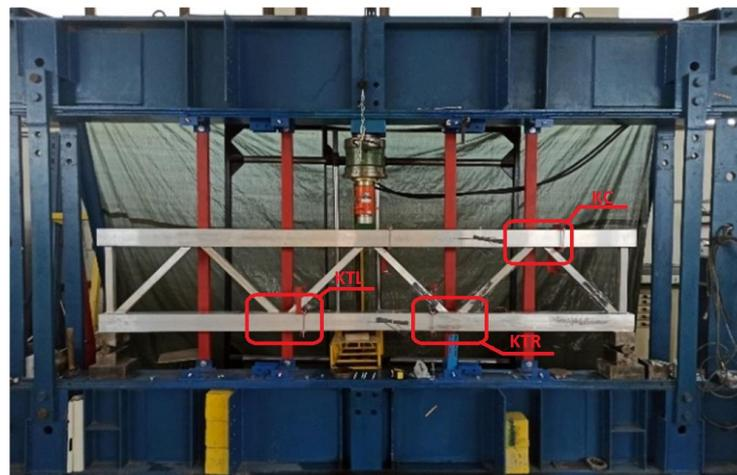
**Figure 4.** Disposition of aluminum lattice girder testing.
