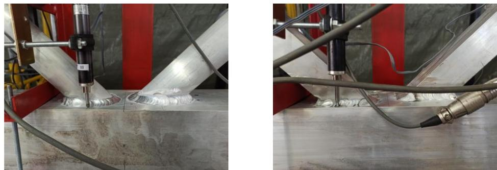
**Figure 7.** K-joint face plastification failure.
