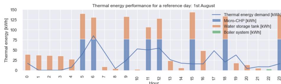
**Figure 6.** Thermal energy performance for a reference day: 1 August.
