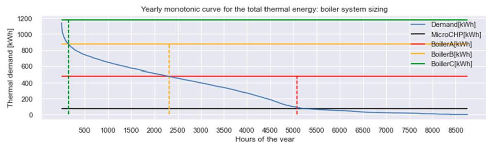
**Figure 3.** The yearly monotonic curve for the total thermal energy: boiler system sizing.
