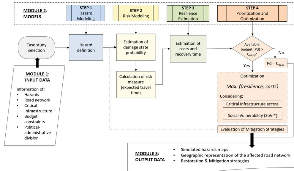
**Figure 1.** Components and framework of the SIGeR-RV tool. Adapted with permission from Ref. [3]. 2023, Sage Journals.
