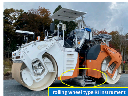
Figure 1. Vibratory roller with rolling wheel-type RI instrument.
