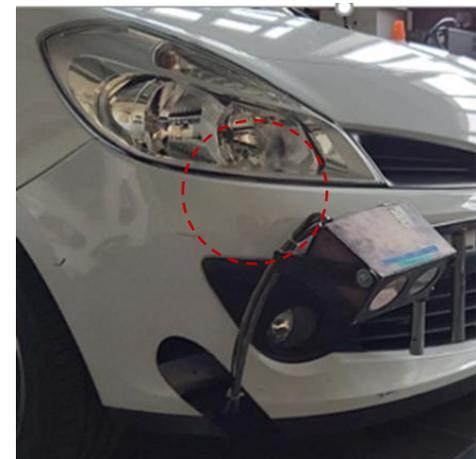
**Figure 2.** Sensors used for the experiments: (a) position of the accelerometers on the front wheel arch (A1 to A4 represent the accelerometers); (b) Aquasens sensor mounted on the test car.
