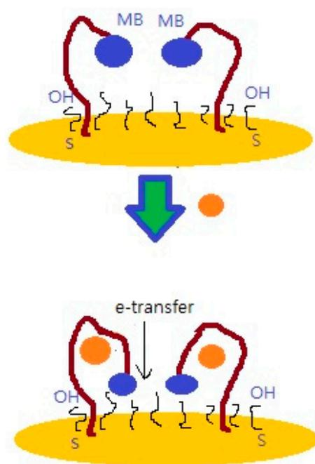
**Figure 1.** A schematical representation of the aptamer conformational changes upon binding to TET. This results in the MB redox tag, coming in close proximity with the gold electrode surface.
