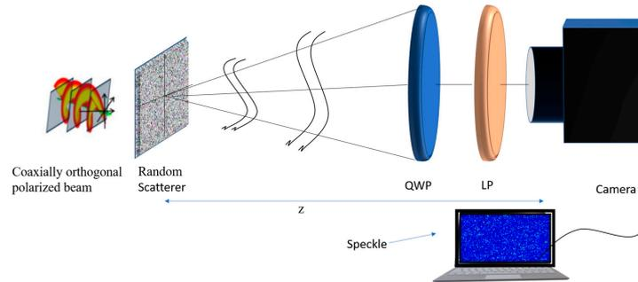
**Figure 1.** Schematic representation of proposed method. QWP—quarter wave plate; LP—linear polarizer. The CCD records intensity speckle patterns at the observation plane. These speckle patterns are used to determine two SPs.
