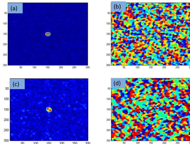
**Figure 2.** Simulation results: (a) amplitude distribution and (b) corresponding phase distribution for vortex beam with a charge of  $l = -1$ ; Experimental results: (c) amplitude distribution and (d) corresponding phase distribution for the vortex beam with  $l = -1$ .
