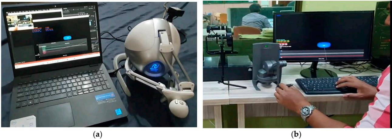
**Figure 4.** Long-distance haptic tele-operation setup. (a) Client-side teleoperator. (b) Server-side teleoperator.
