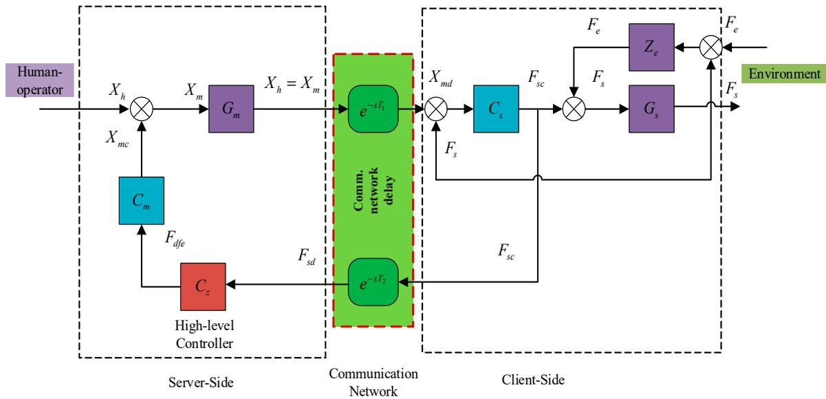
**Figure 1.** Control architecture of the bilateral haptic teleoperation framework.
