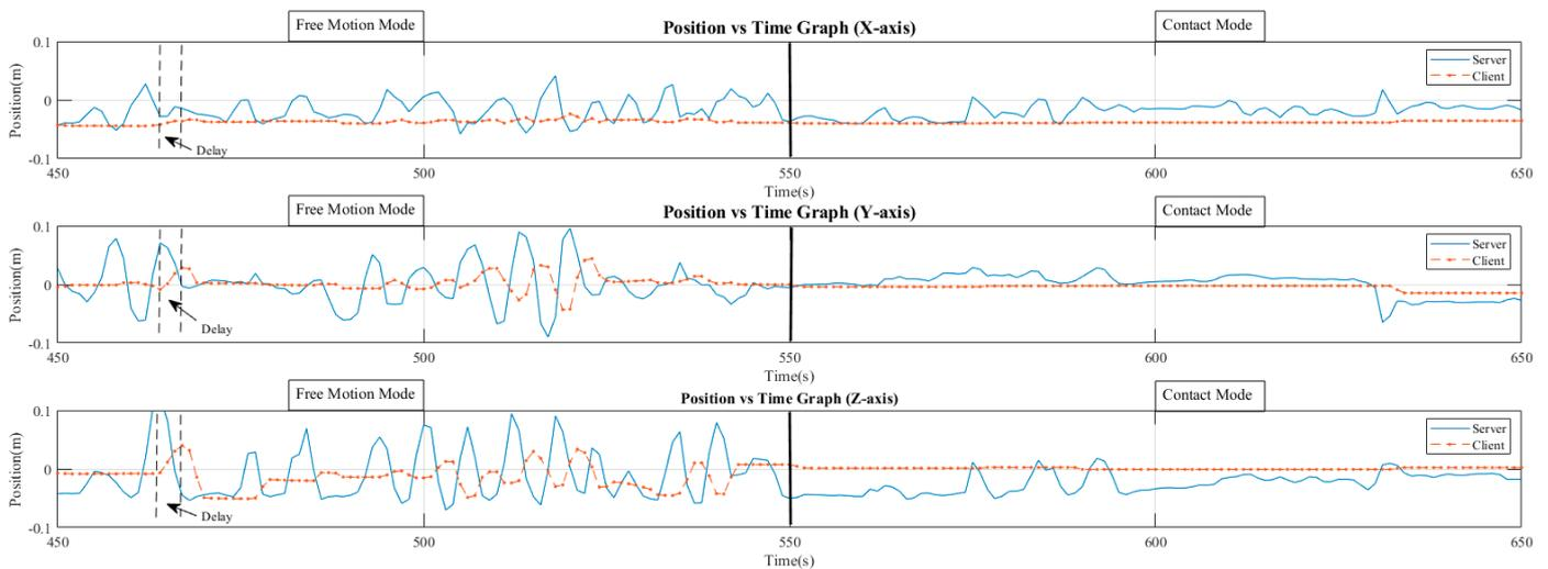
**Figure 5.** Server–client position data of long-distance (7000 km approx.) delayed haptic teleoperation.
