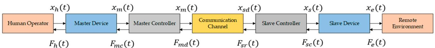
**Figure 2.** Block diagram of bilateral haptic teleoperation (position–force (PF) architecture).
