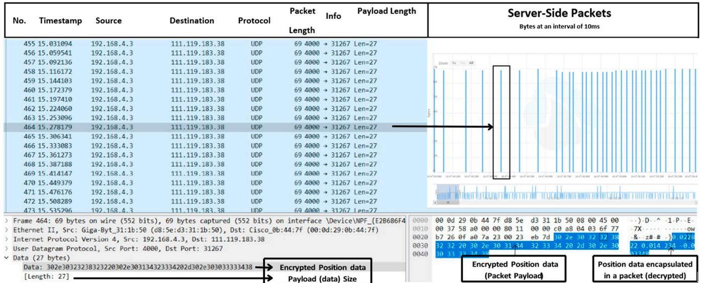
Figure 3. Real-time haptic data packets containing (x, y, z) position coordinates (captured at the server end).
