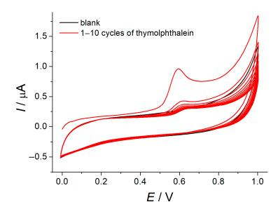
**Figure 1.** Electropolymerization of 10  $\mu$ M thymolphthalein at the MWNT/GCE in phosphate buffer pH 7.0.  $v = 100 \text{ mV s}^{-1}$ .
