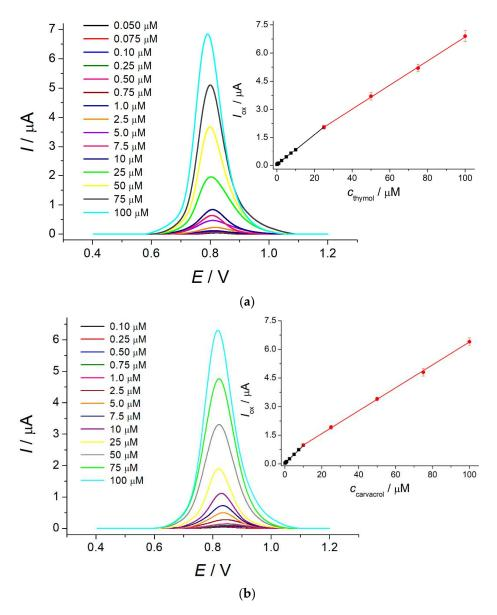
**Figure 2.** Differential pulse voltammograms of isopropylmethylphenols at the polythymolphthalein/MWCNTs/GCE in Britton–Robinson buffer pH 2.0: (**a**) thymol; (**b**) carvacrol.  $\Delta E_{\text{pulse}} = 100 \text{ mV}$ ,  $t_{\text{pulse}} = 25 \text{ ms}$ , and  $v = 20 \text{ mV s}^{-1}$ . Inserts are the corresponding calibration graphs.
