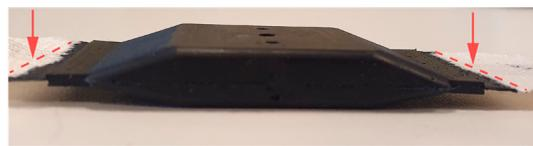
**Figure 1.** Final sample encapsulation; red markings highlight the transition/high-stress areas.
