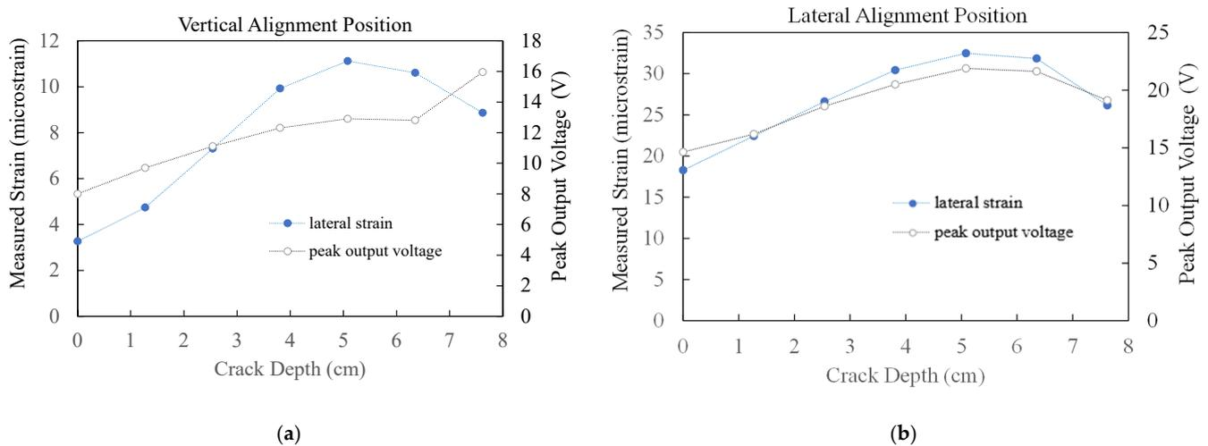
**Figure 4.** Measured lateral strain (along the  $x$ -axis) and peak piezoelectric-based sensor output in response to the depth of the bottom-up crack when the dynamic load moving velocity equals 25 km/h: (a) sensor is vertically aligned (along the  $y$ -axis); (b) sensor is laterally aligned (along the  $x$ -axis).
