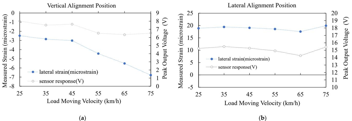
**Figure 3.** Measured lateral strain (along the x-axis) and peak piezoelectric-based sensor output in response to the dynamic load moving velocity when there is no bottom-up crack existing in the asphalt concrete pavement (crack depth = 0 cm): (a) sensor is vertically aligned (along the y-axis); (b) sensor is laterally aligned (along the x-axis).
