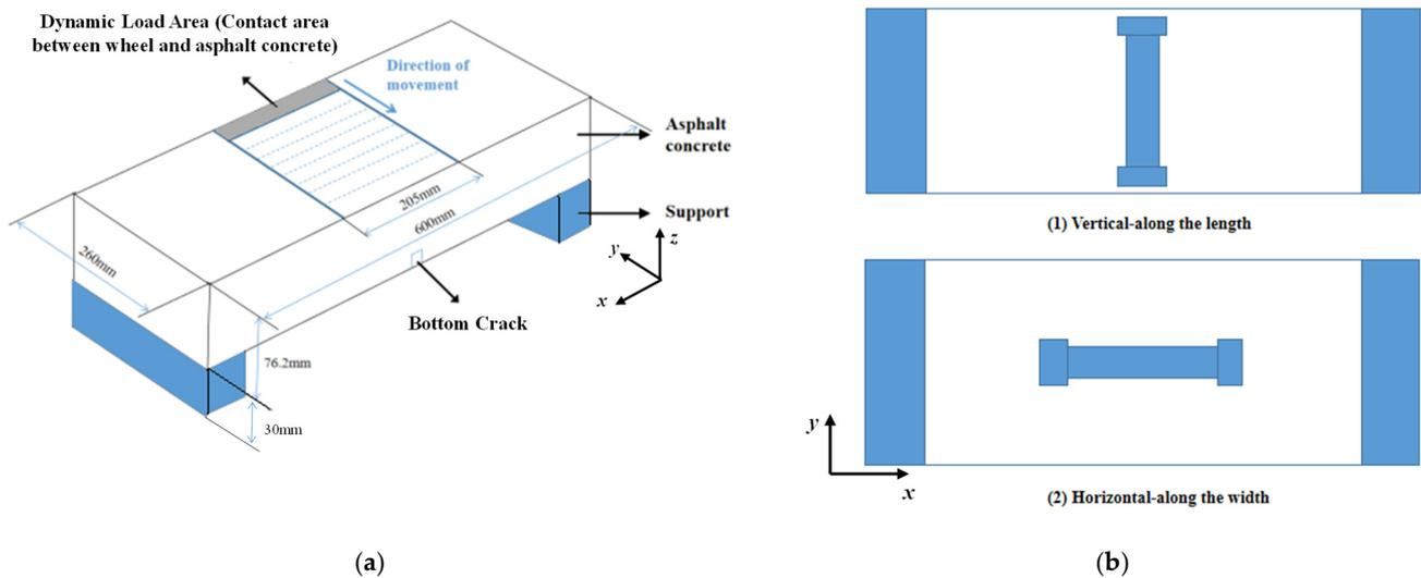
Figure 2. (a) Schematic of the numerical model of a dynamic load passing through the road surface. (b) Bottom view of the numerical model for showing sensor alignment.
