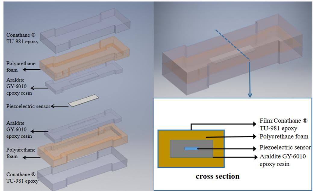
Figure 1. Configuration of the strain sensor.
