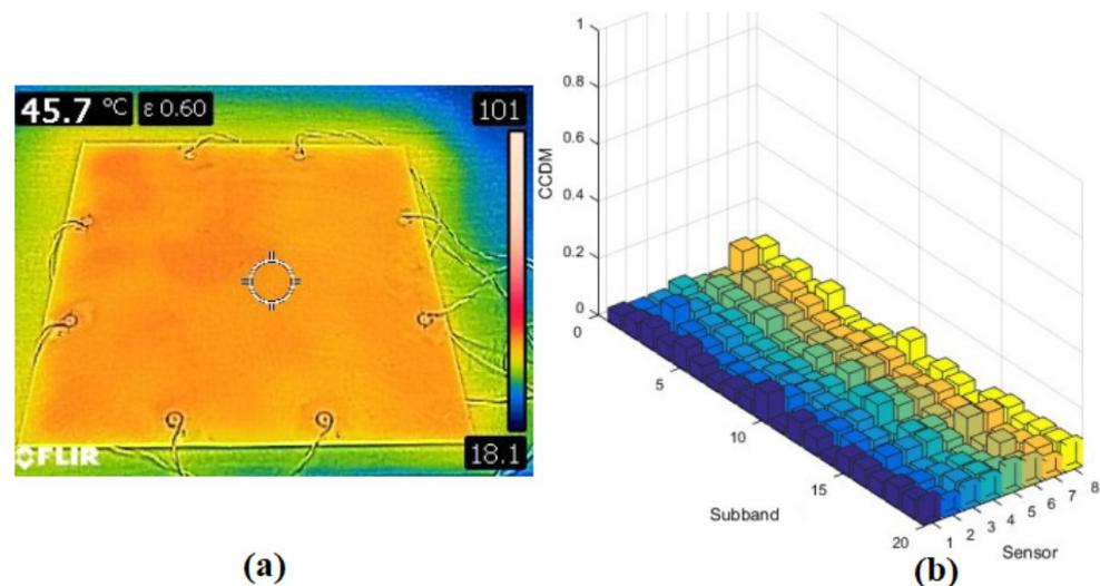
**Figure 3.** (a) Thermal image of the uniformly heated structure; (b) CCDM indices calculated after compensation with the EFS method.
