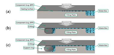
**Figure 4.** Working principles of the sealing systems developed: (**a**) without additional sealing element, (**b**) sealing by means of an O-ring, (**c**) sealing by means of a combination of O-ring and support ring.
