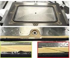
(**b**) O-ring flows into segment separation if gap is present
