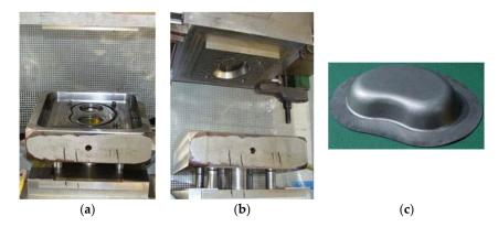
**Figure 2.** (**a**,**b**) Tool for passive hydroforming; (**c**) test components applied with tool (material: DX54D steel, wall thickness 0.6 mm), according to [7].
