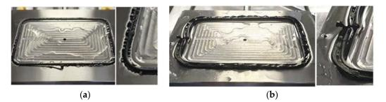
Figure 7. O-ring sealing-failure cases: (a) O-ring starts to flow and (b) O-ring seal failure at 200 MPa.
