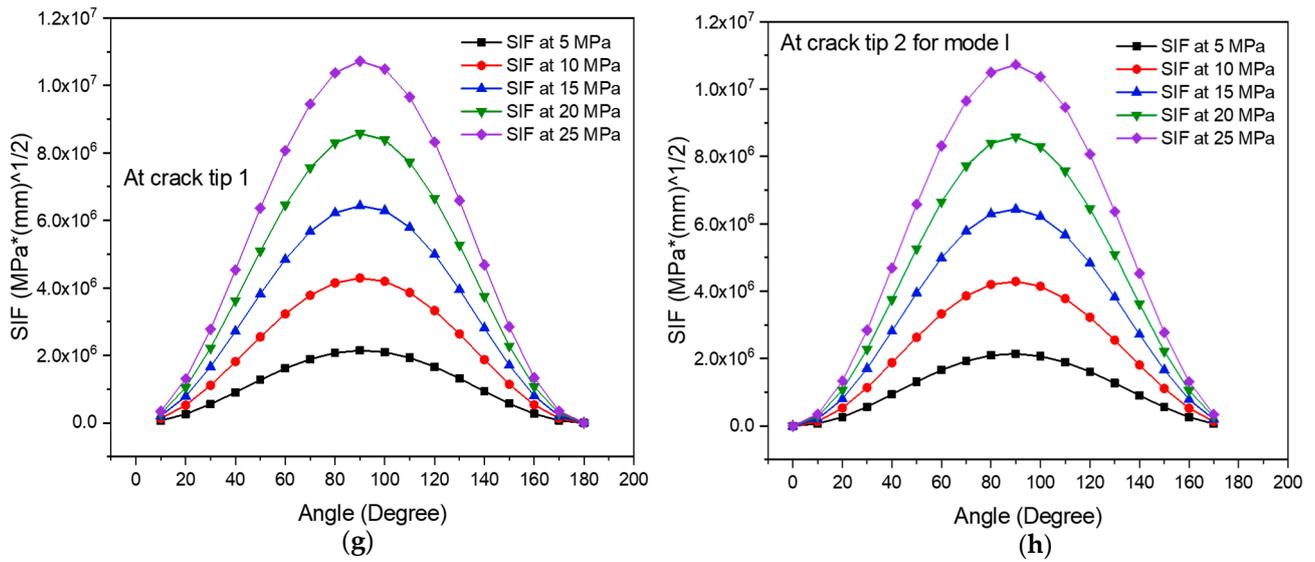
**Figure 2.** The variation of crack opening displacement with angle and loads (a) The variation of crack sliding displacement with inclination and loads (b) The SERR for mode I at crack tip 1 (c) The SERR for mode I at crack tip 2 (d) The SIF for mode II at crack tip 1 (e) The SIF for mode II at crack tip 2 (f) The SIF for mode I at crack tip 1 (g) The SIF for mode I at crack tip 2 (h).
