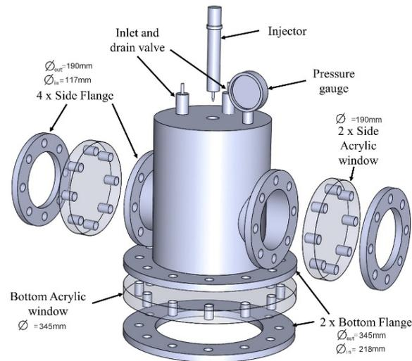
**Figure 1.** Schematic diagram of CVSV with fabrication details.
