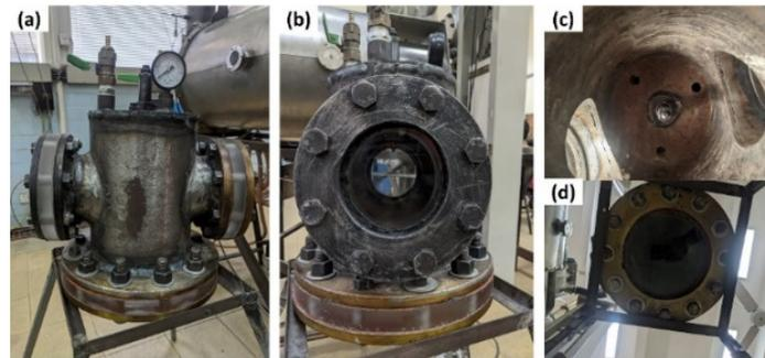
**Figure 3.** Various orientations of CVSC. (a) Sealed CVSC rested on a stand, with pressure gauge, injector and drain valves on the top, (b) Side view of CVSC, (c) Inside view of CVSC from the bottom window and (d) Bottom view of CVSC.
