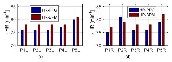
**Figure 4.** Summary bar-graph comparison of mean HR values determined from PPG signals and measured by a BPM device: (**a**,**b**) from four fingers of L/R hands and both ear lobes using the *FRS* and *ECS* sensors; (**c**,**d**) from five fingers of L/R hands using the *REFS* sensor; tested male person JP.
