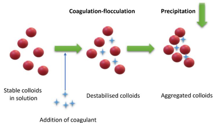
**Figure 2.** Coagulation-flocculation-decantation scheme.
