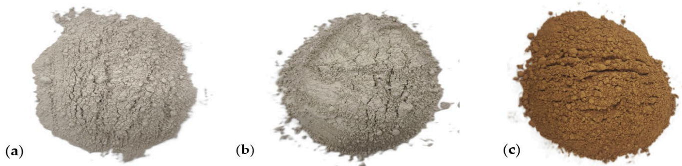
Figure 1. Supplementary cementitious materials in powder form: (a) recycled concrete powder (RCP); (b) limestone powder (LF); (c) recycled clay brick powder (RCBP).
