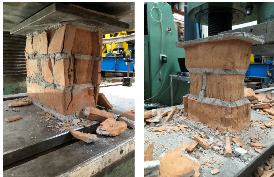
Figure 5. Specimen after failure.
