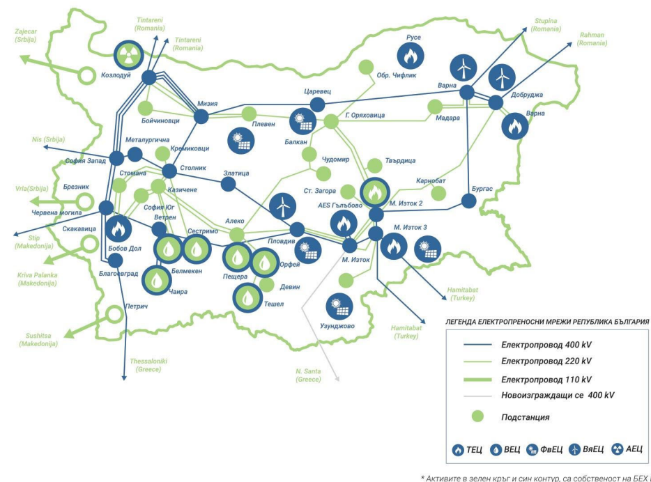
Figure 1. Map of the Bulgarian energy grid showing main transmission lines along with main power plants. Note: The energy ring is formed to provide redundancy. Note: Names on the map are power plants with pictures depicting the primary energy source. Green dots are substations, while power lines are colored as follows: 400 kV—blue, 220 kV—green (thin line), 110 kV—green (thick line), 400 kV (under construction)—light purple. Names of power stations and power lines are in italics in Cyrillic (irrelevant to the study). Glyph icons in the bottom of the legend table are as follows from left to right—Thermal Power Plant, Hydroelectric Power Plant, Photovoltaic Power Plant, Wind farm, Nuclear Power Plant [4].
