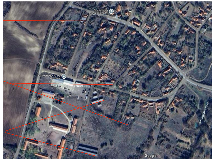
Figure 4. Azimuth of several “south” facing PV plants. The red lines indicate the real azimuth as opposed to the claimed south. The image is perfectly oriented, with south being the horizontal boundary of the image.
