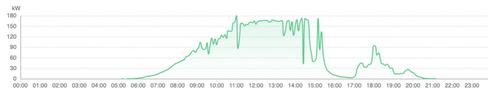
Figure 3. Production of a 200 kWp PV plant on a cloudy day.
