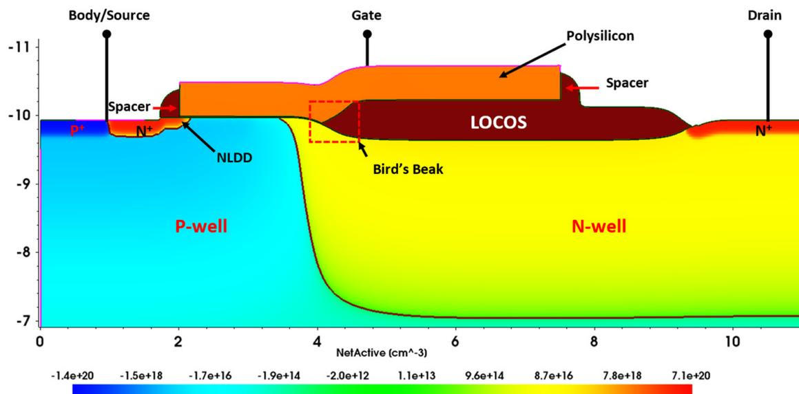
Figure 2. Final structure net doping profile.
