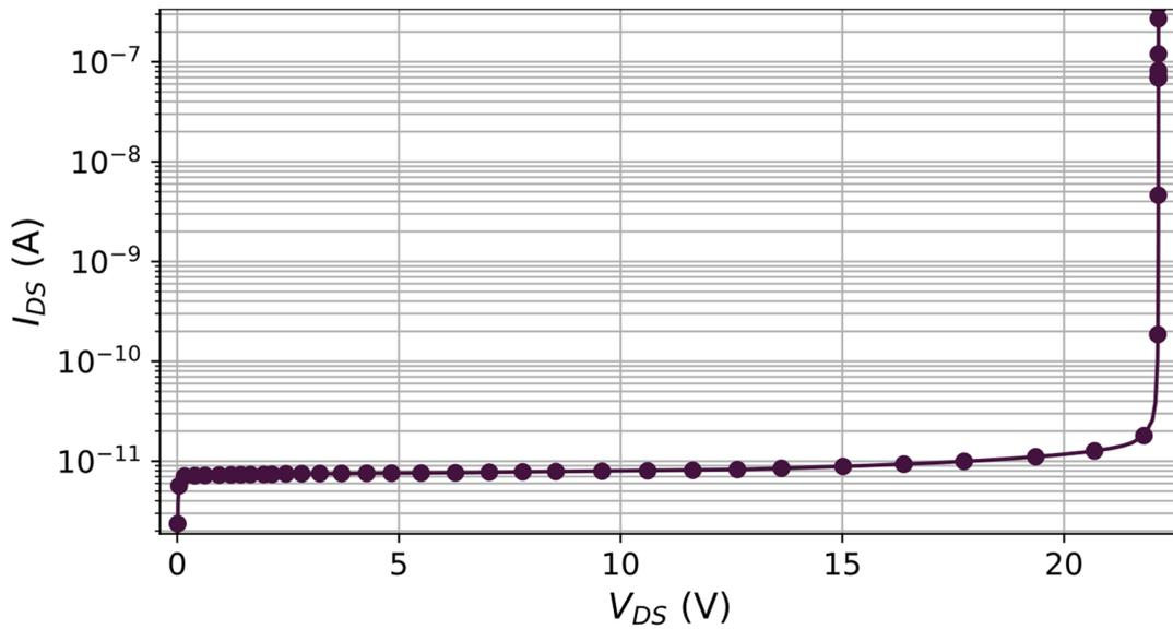
Figure 4. Off-state breakdown characteristic of the LDMOS.
