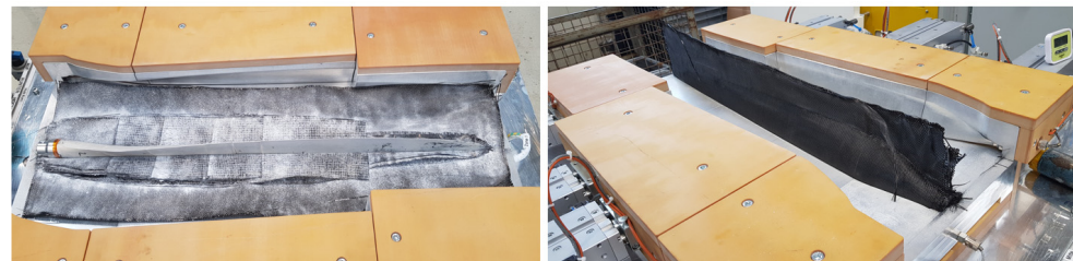
Figure 4. Fiber layup and salt core in the preforming tool for sequential draping (left) and final preform for subsequent processing in HP-RTM (right).
