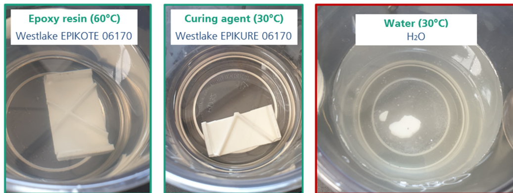
Figure 1. Salt core samples consisting of potassium chloride (KCl) and sodium carbonate ( \text{Na}_2\text{CO}_3 ) in the chemical compatibility test and solving test with water.
