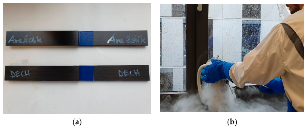
Figure 2. CFRP materials for the SMA strain sensors (a) and their tests in cryogenic environment (b).
