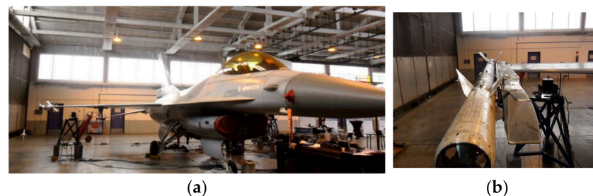
Figure 1. Ground Vibration Testing experimental setup. (a) F-16 aircraft prepared for the test; (b) the dummy payload on the tip of the right wing (retrieved from [13]).
