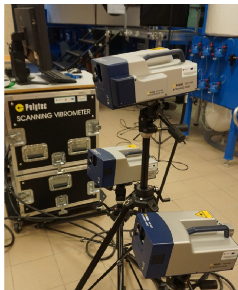
Figure 1. PSV-400-3D scanning laser vibrometer with three measuring heads. The geometry scanning unit is installed on the upper head.
