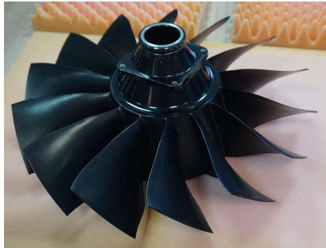
Figure 3. Measurement object—rotor of the first stage of the DGEN 380 engine compressor.
