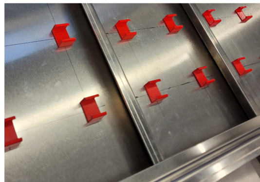
Figure 1. Mounting brackets for energy harvesting resonators attached to a stiffened plate as a model for the airframe.
