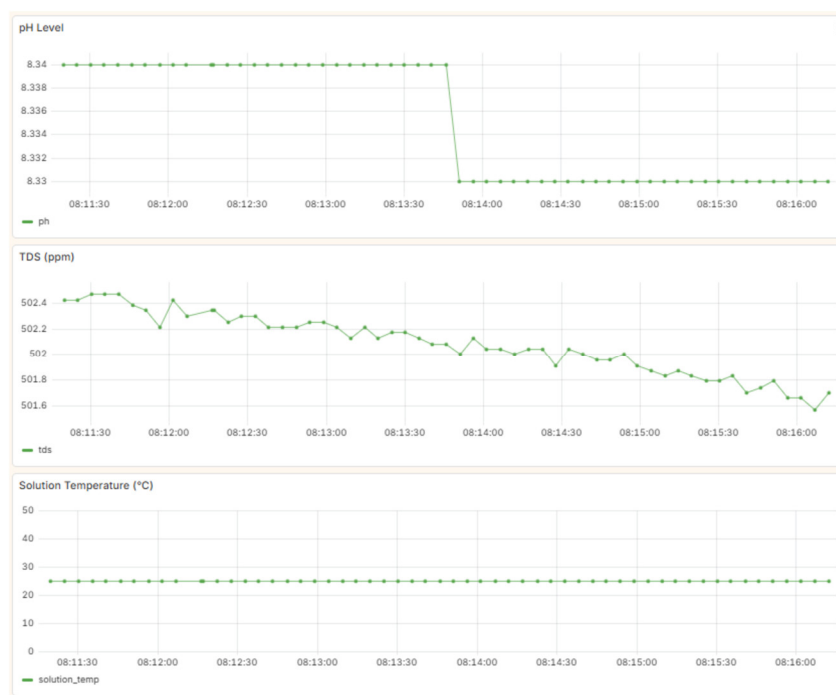
Figure 7. Grafana dashboard visualization of a 10-min time-series excerpt showing pH, TDS, and nutrient solution temperature from InfluxDB data.
